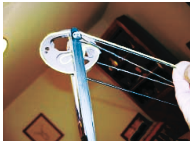
Photo 5 Measuring end loop serving length . . .
