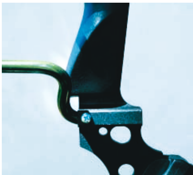
Figure 3. Cable Guard Mounting. Once the cable guard epoxy glue has cured, cross drill and insert an 8-32 machine screw to prevent future rotation of the rod.
