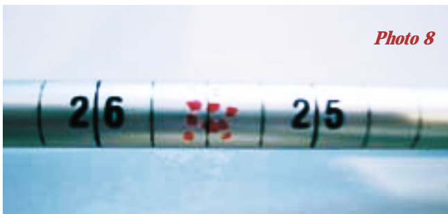
Photo 8 View of Draw Variance using Triple Tape System.
