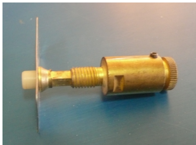
This version had a plate for a stick on arrow rest and a square shaft to keep it from rotating. A good idea that wasn't well received.
