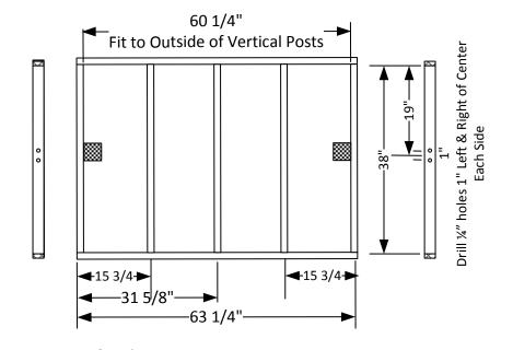
Cut List: 5ea 2" x 4" x 38" PT Studs 2ea. 2" x 4" x 63 ¼" PT Headers Attach with 3 ½" Deck Screws
