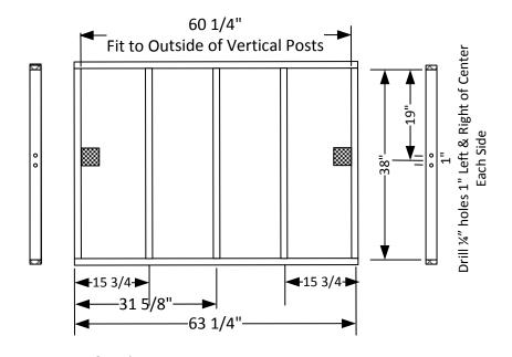
Cut List: 5ea 2" x 4" x 38" PT Studs 2ea. 2" x 4" x 63 ¼" PT Headers Attach with 3 ½" Deck Screws
