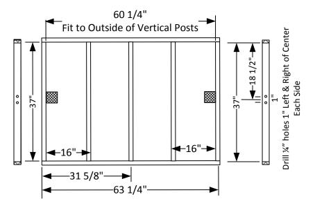
Cut List: 5ea 2" x 4" x 37" PT Studs 2ea. 2" x 4" x 63 ¼" PT Headers Attach with 3 ½" Deck Screws
